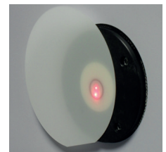
Sapphire sample: The two beams are visible by transparency
