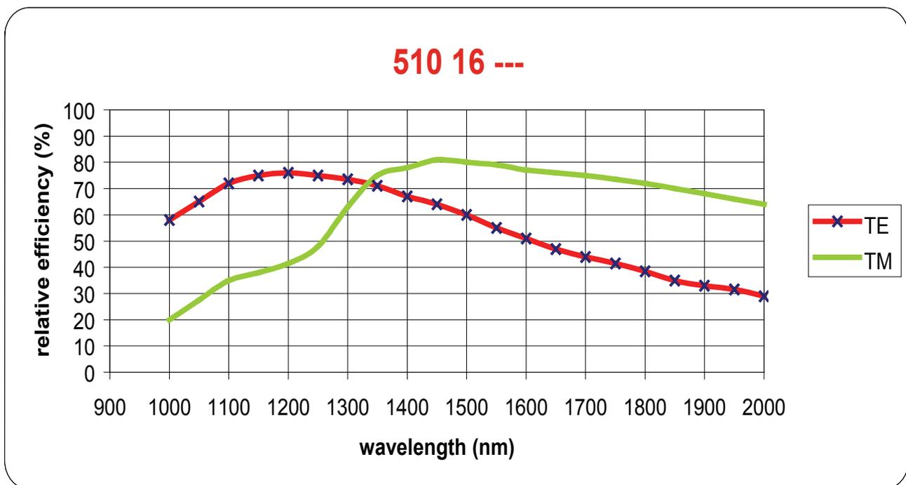
This efficiency curve should be used as reference only and does not imply any guarantee on actual performance. Actual performance of the grating will depend on several variables including the usage geometry and the coating. Efficiency curves labeled as "Theoretical" are calculated estimates of performance based on groove profile.
