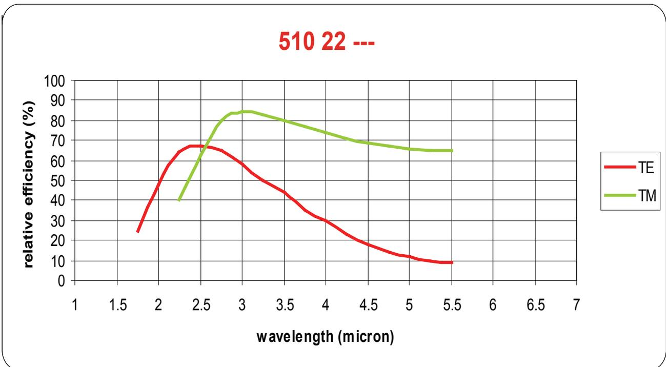
This efficiency curve should be used as reference only and does not imply any guarantee on actual performance. Actual performance of the grating will depend on several variables including the usage geometry and the coating. Efficiency curves labeled as "Theoretical" are calculated estimates of performance based on groove profile.
