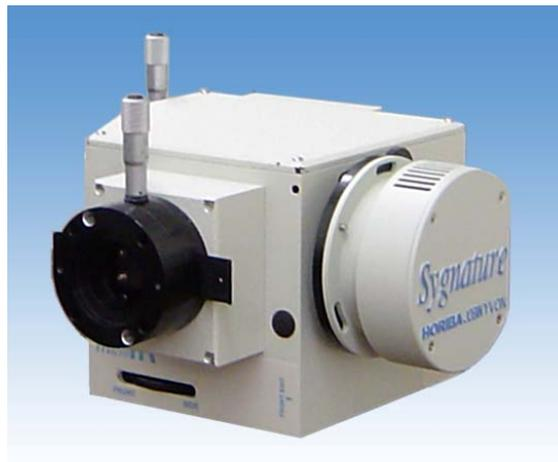
The automated MicroHR equipped with side exit option and Signature CCD
