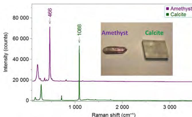
Figure 1: Raman spectra of amethyst and calcite crystals.
