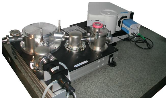
H20-UVL used in a VUV fluorescence setup
