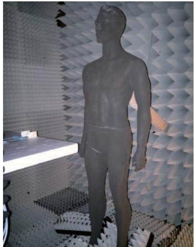
Figure 2 Metal-coated mannequin and antennas used in the measurement.
