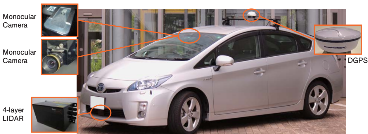
Figure 1 Equipped sensors for experimental vehicle
